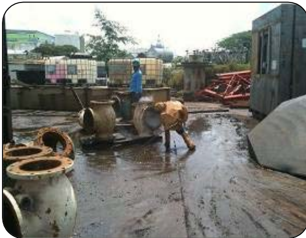
Hydro-jetting and Sandblasting of Valves in Kim Heng Yard
