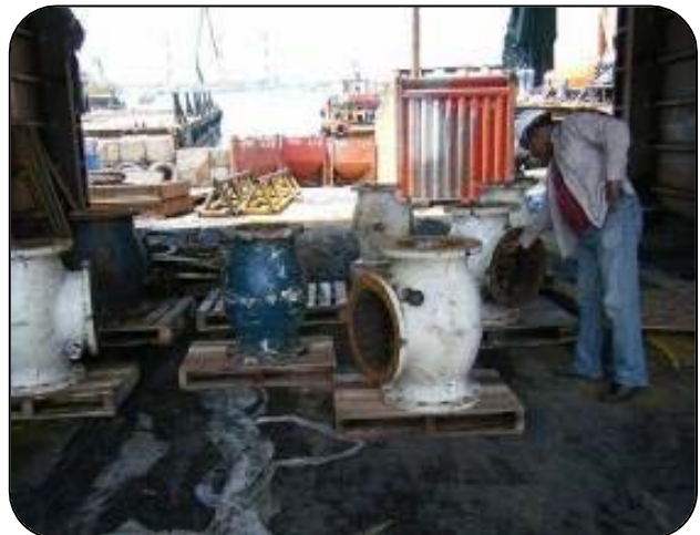
Hydro-jetting and Sandblasting of Valves in Kim Heng Yard
